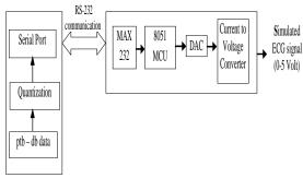
Fig 1: Block Diagram of the system.
