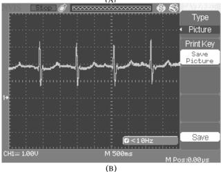
**Fig 5:** Experimental Results (A) Hardware setup for ECG simulator, (B) DSO output of Simulated ECG signal for p2/s0016\_v3.
