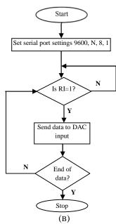
**Fig 3:** (A) Flowchart for serial data transmission using MATLAB (B) Flowchart of serial to parallel data conversion at embedded system.
